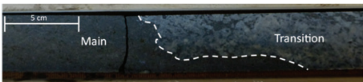
Figure 5. Drill hole DDH64 at 5.18 m, contact between Main Zone and Transition Zone material.
