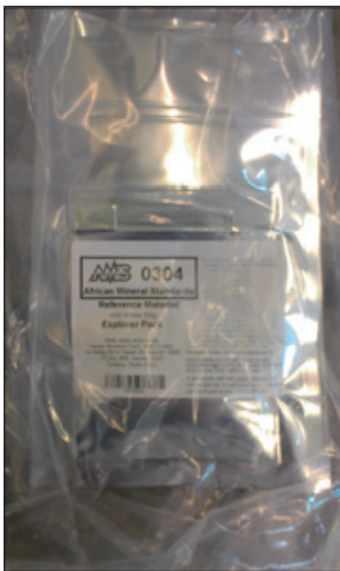
Figure 8. AMS certified Standard Reference Material used during recent assay of 2012 drilling by Kodal.
