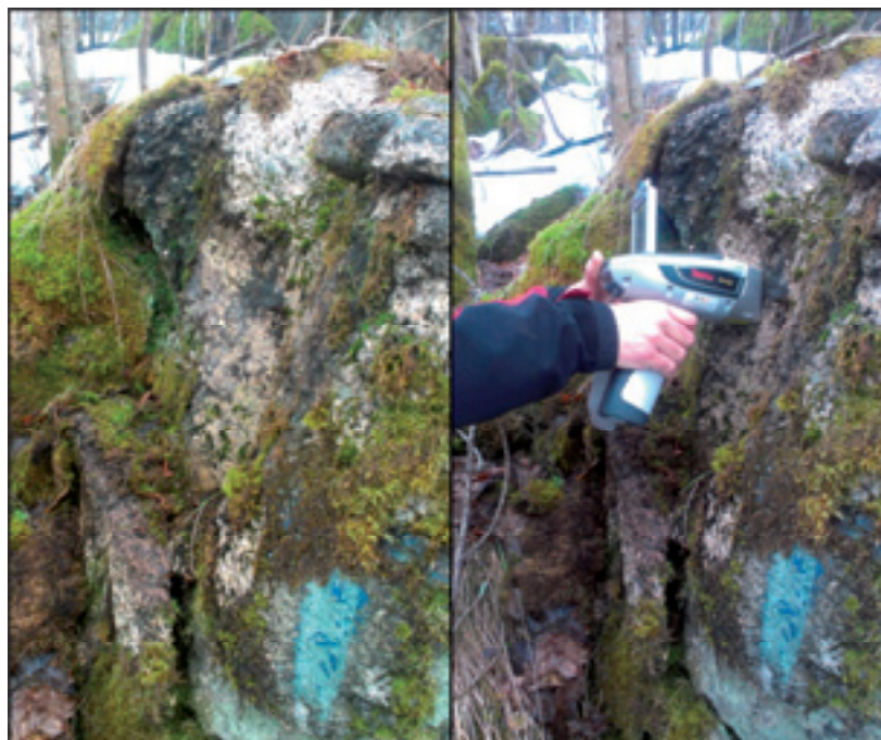
Figure 14. Mineralised outcrop of larvikite at the Kodal Project. Handheld XRF (Niton XL3t) returned low level Fe, P and Ti mineralisation at concentrations similar to those found in the hanging wall “transition” zone.
