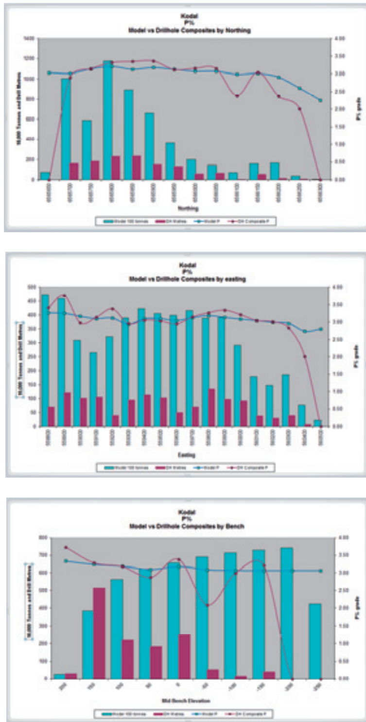
Figure 10. Swath Plots of the 2013 MRE block model (P%), with slices through the model in the Northing (upper plot), Easting (central plot) and RL (lower plot) directions, showing grade smoothing.
