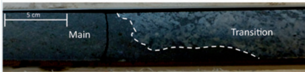
Figure 5. DDH64 5.18 m, contact between Main Zone and Transition Zone material.
