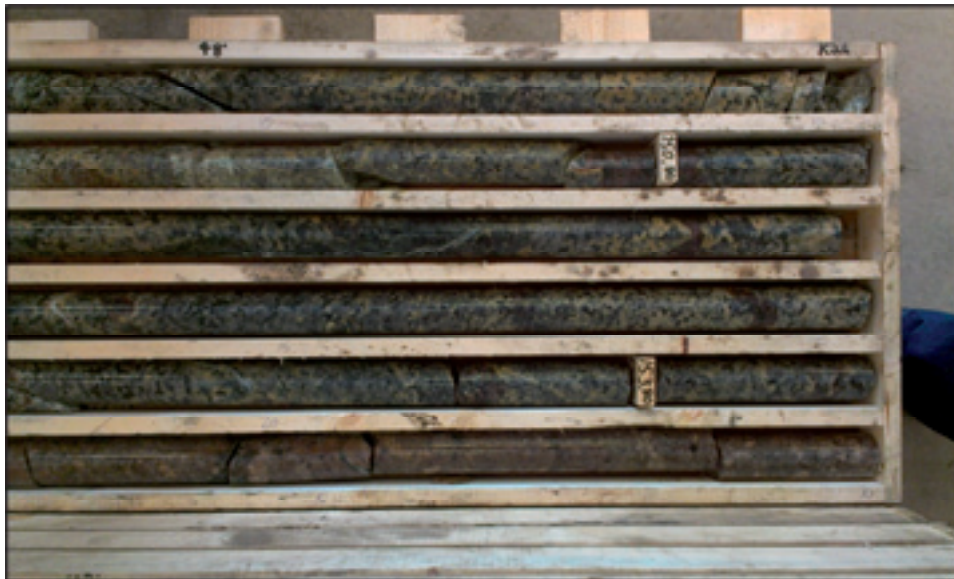
Figure 4. Core from BH63, showing the Jacipurangite/Larvikite footwall contact. Core from this hole was reviewed against hardcopy cross sections and summary logs of hole BH47, which it twinned.
