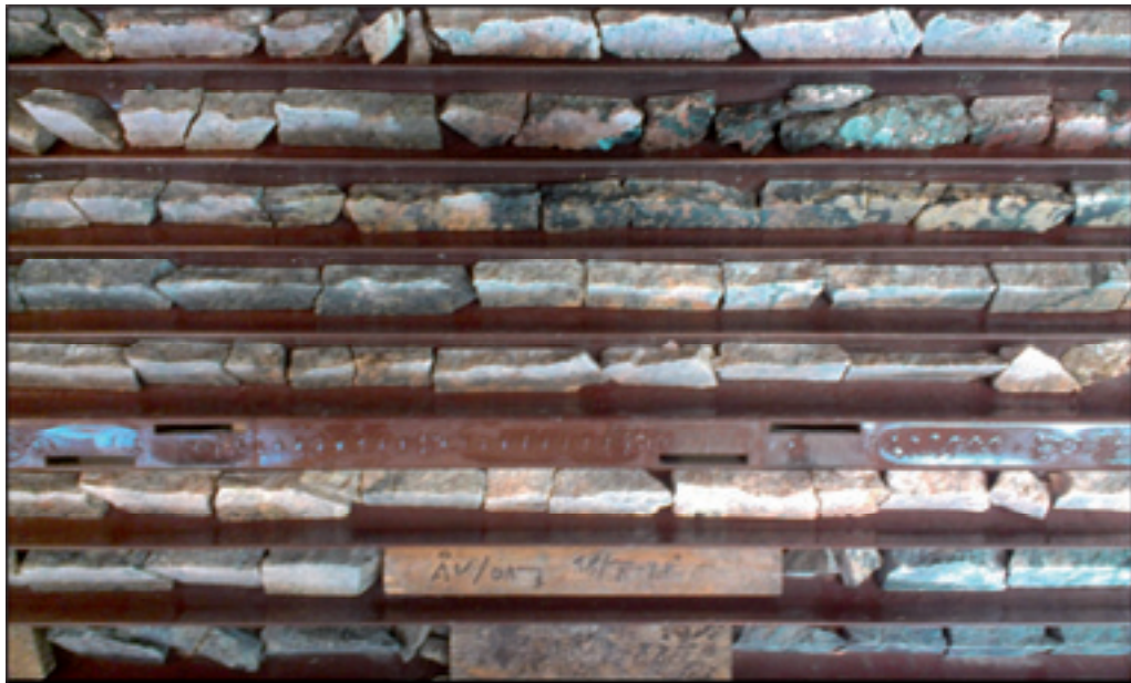
Figure 6. Core from BH 44, recently sampled by Kodal (quarter core).
