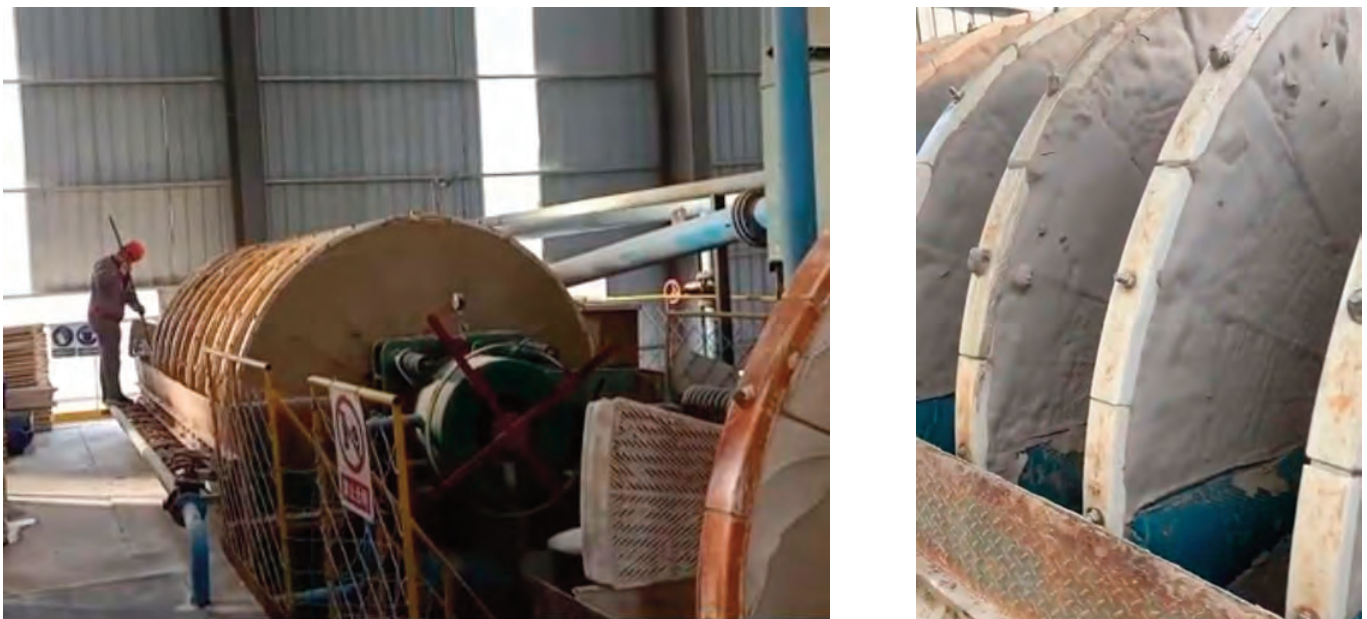
Figure 6: Flotation product undergoing filtration for reduction of moisture content to <5%
