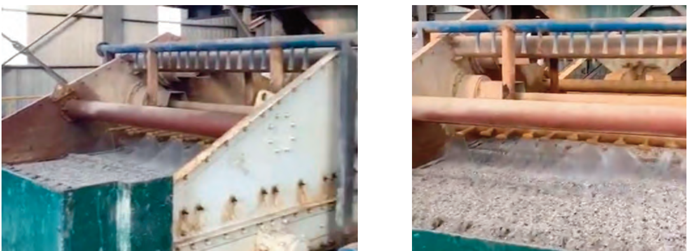
Figure 5: Primary sizing screen separating coarse DMS feed material from the finer Flotation feed material
